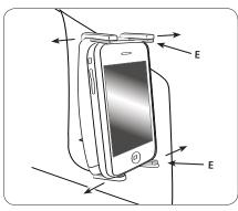
Step 1. If necessary, adjust the support legs (E) on top and bottom by sliding them laterally to avoid any buttons or ports that may be on your phone.
